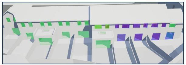
Image 6.5: Window Map illustrating compliance to NSL daylight test
