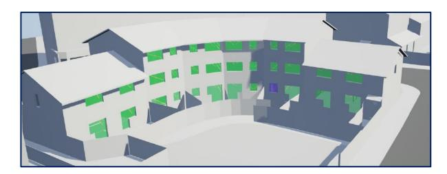
Image 6.3: Window Map illustrating compliance to NSL daylight test
