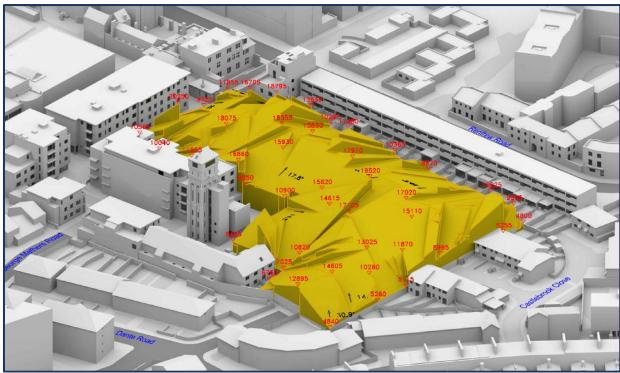
Image 3.3 - 3D representation of the development capacity of the Site if the effects fully adhered to the BRE Guidelines- view looking south west
