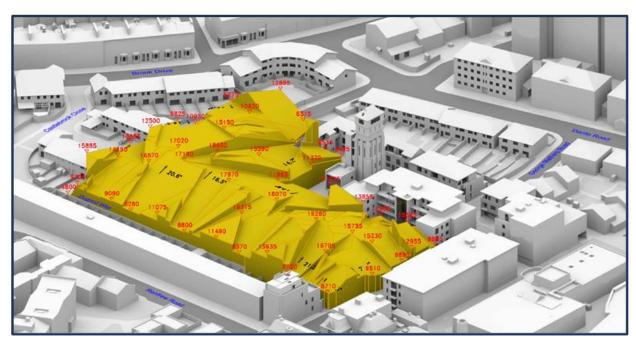
Image 3.2 - 3D representation of the development capacity of the Site if the effects fully adhered to the BRE Guidelines- view looking north east
