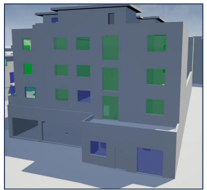
Image 6.18: Window Map illustrating compliance with alternative VSC target
