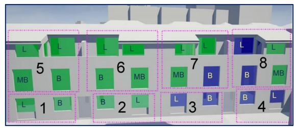
Image 6.16: Window Map illustrating compliance with alternative VSC target
