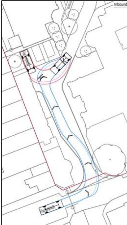
Figure 62 - Tracking of a servicing vehicle entering the site in forward gear. The vehicle would also be able to exit in forward gear
