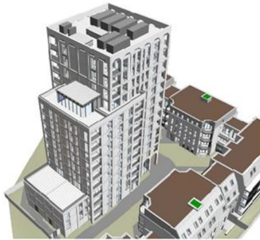
Figure 34 - Massing of Block A to address daylight impacts. Note the storey heights are now 3, 4/5 then 14.
