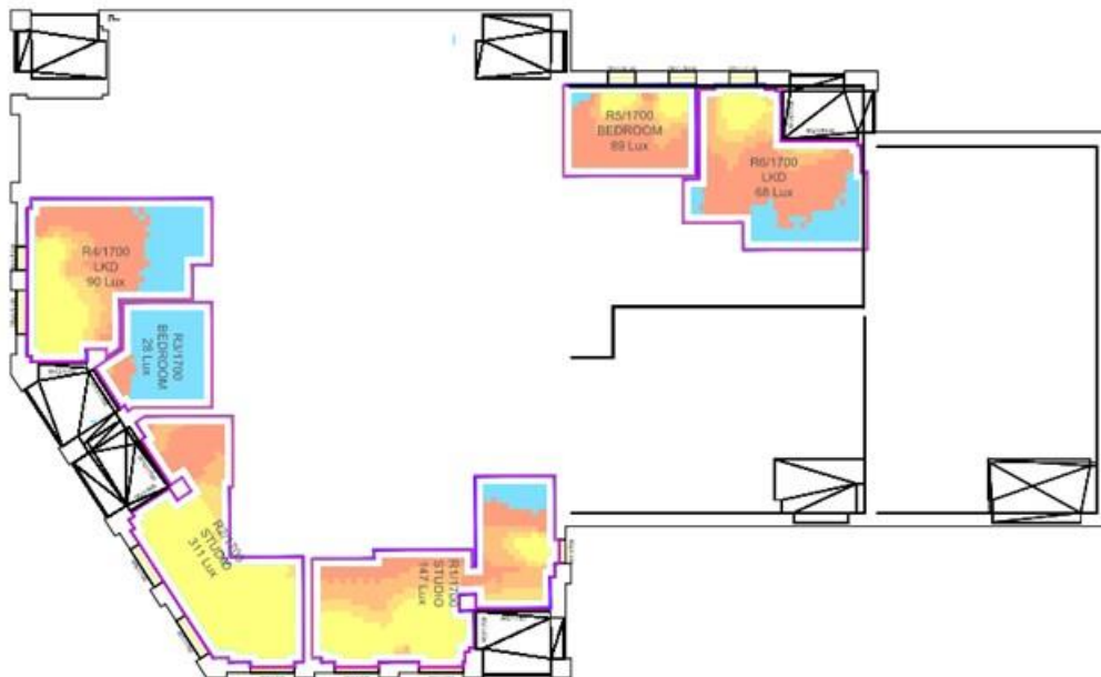
Figure 29 - Ground floor plan (top) and first floor plan (bottom) showing illuminance levels. Yellow
