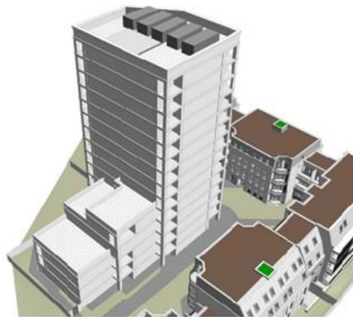
Figure 34 - Massing of Block A to address daylight impacts. Note the storey heights are now 3, 4/5 then 14.
