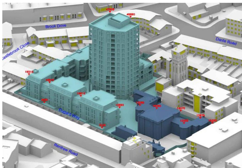
Figure 7 - 3D massing model of the proposed development. The retained Master's House building is in dark blue
