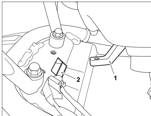
**7** Lower the front of the seat ensuring the seat retaining peg (1) is aligned correctly with rider seat retaining bracket (2) and the seat latch assembly (3), as shown. Press the front of the passenger seat down to engage in the seat latch.
