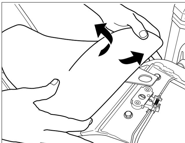
**4** Fit the touring rider seat to the motorcycle ensuring the front seat retainer (1) locates correctly in the motorcycle frame (2).
