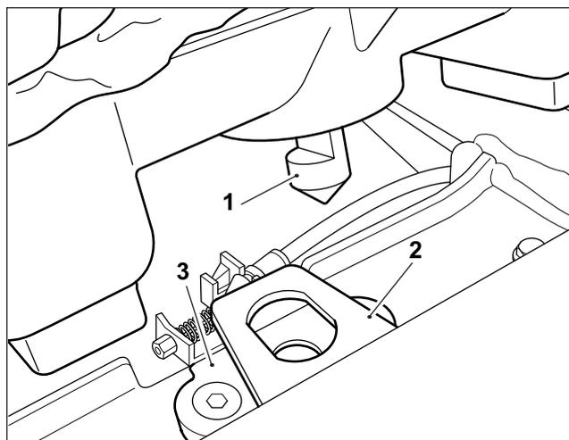
**WARNING:** Pull the front of the seat upwards to check the seat is securely attached to the motorcycle. If the passenger seat is not correctly secured to the motorcycle it may allow movement or possible detachment of the rider or passenger seats while riding. A loose or detached seat may cause the motorcycle to become unstable and result in an accident.
