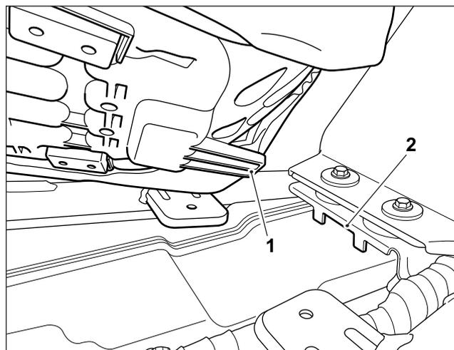
**5** Lower the rear of the seat ensuring the seat retaining bracket (1) is aligned correctly with the seat latch assembly (2), as shown.
