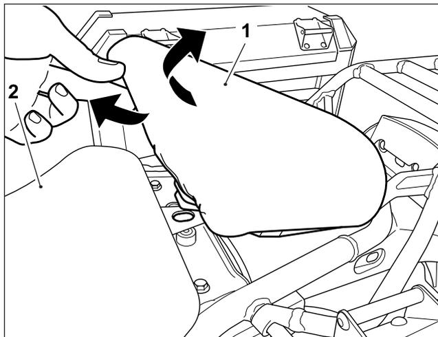
**3** Lift the rear of the original rider seat and slide the seat towards the rear of the motorcycle to remove, as shown. Retain the original rider seat for reuse if the accessory touring seat is removed.
