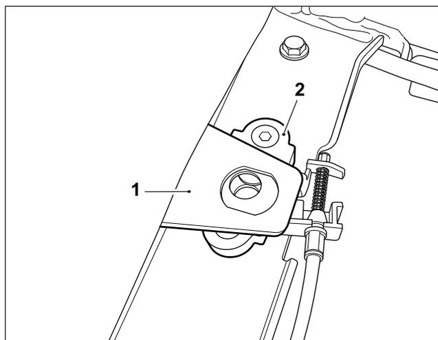
**6** Refit the passenger seat to the motorcycle ensuring the retainer (1) on the rear of the seat locates correctly in the motorcycle frame (2).
