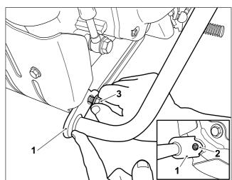
**3** Align the top mounting of the left hand engine guard (1) with the top engine mounting location and refit the original fixing (2), as shown.
