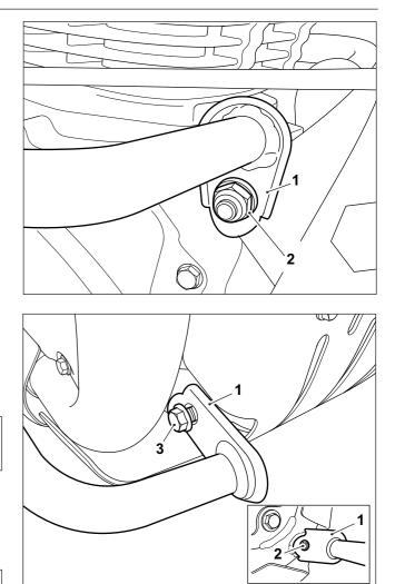
**6** Align the bottom mounting of the engine bar (1) with the with the mounting point on the motorcycle frame (2). Fit an M8 x 12mm fixing (3) from the kit. Tighten the fixing to **16Nm**.
