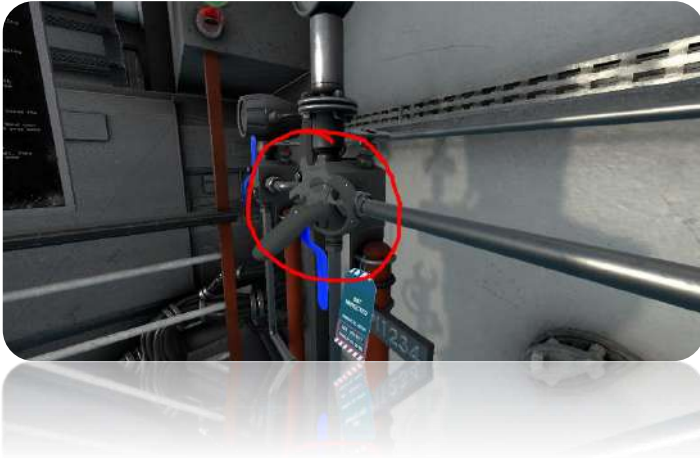
Figure 11 - The use of the inspection gauge against the pipe fitting, confirming the nut is not the source of the fault.
