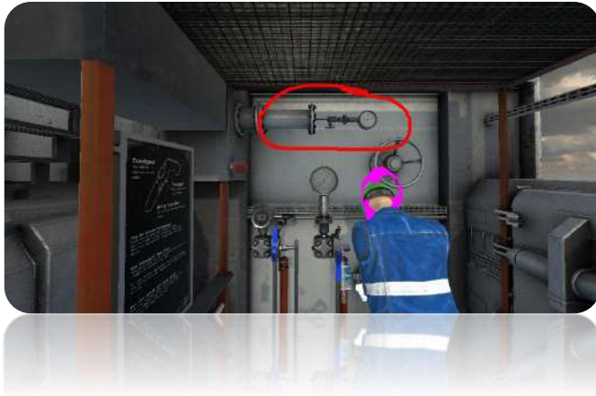
Figure 15 - The trainee should identify the pipe gauge is not adequately attached to a work surface and notify the System Manager when prompted: "There is a heavy pressure gauge on the end of a thin tube above the fault area".
