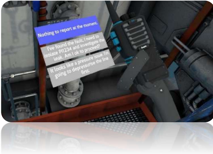
Figure 5 - The trainee should report the fault to the system manager using Option 2: "I've found the fault, I need to isolate PI1234 and investigate the leak. Am I ok to proceed?"
