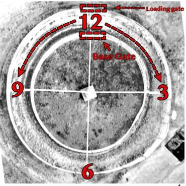
8. This process will be repeated on the opposite side from the 6 o'clock position to the 9 o'clock position and from the 6 o'clock position to the 3 o'clock position. Once this is completed, you should be able to manually spin your walker completely around while clearing all panels. Once they are properly clearing, which might take small adjustments, you will then secure the inner circle panels with stakes provided through the hole in the bottom of each panel.
