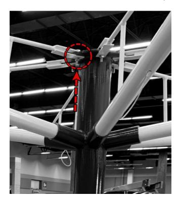
4. Attach hanging dividers to each arm using included hardware. The chain pattern will be a "N" as pictured. Make sure after all panels are installed, using a level, that they are level. The top of the divider should be approximately 6 feet from the ground.
