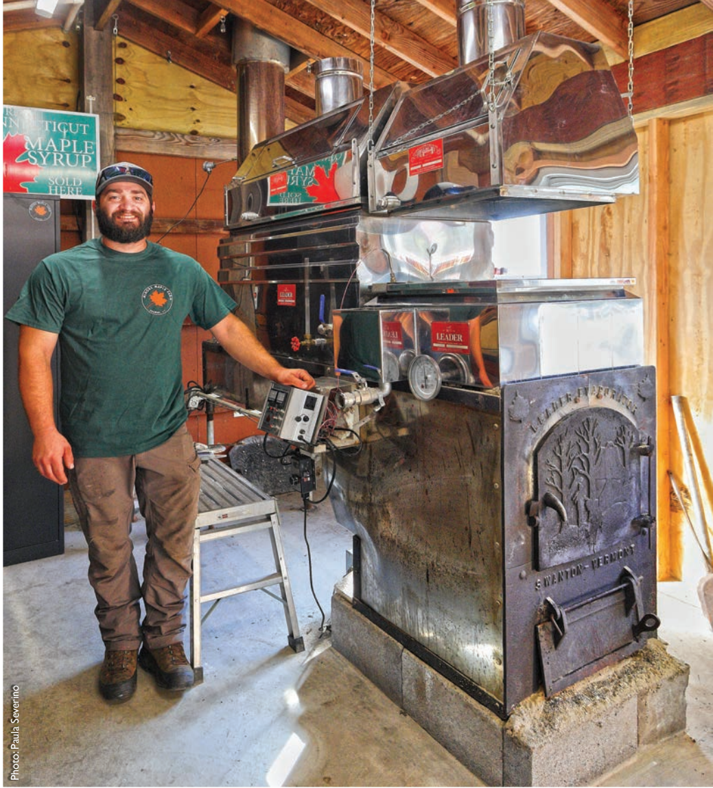
Chris Minore with the evaporator machine where raw sap gets boiled, which concentrates the natural sugars and creates the thick, sweet syrup.
