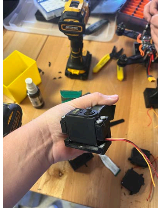
Shows the servo sitting in the housing
