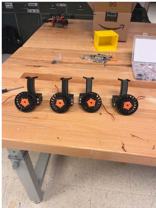
Attached the tire to the rims. Then screwed the wheel into the servo
