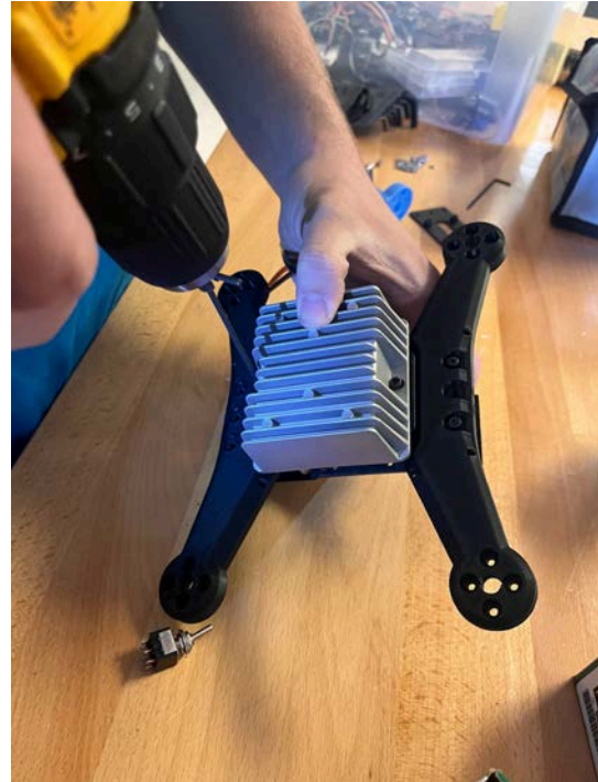
The new buck converter was installed to handle the currents from the servos.
