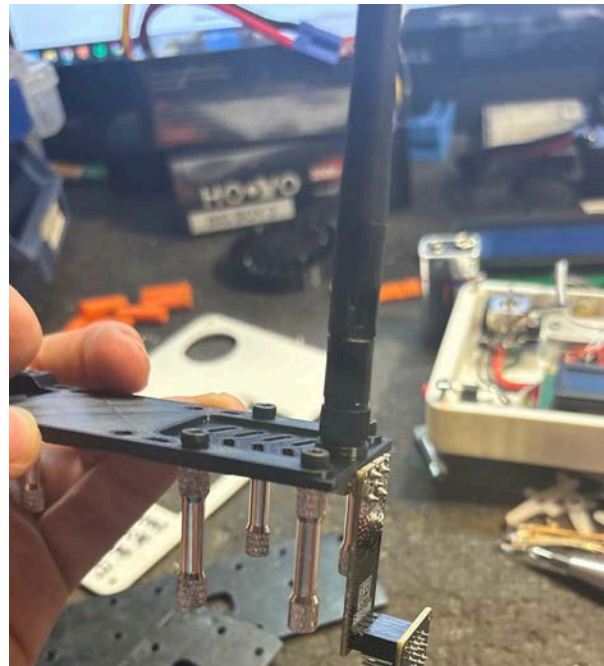
Begin to screw vertical posts and NRF into the top plate to make sure the screw holes fit
