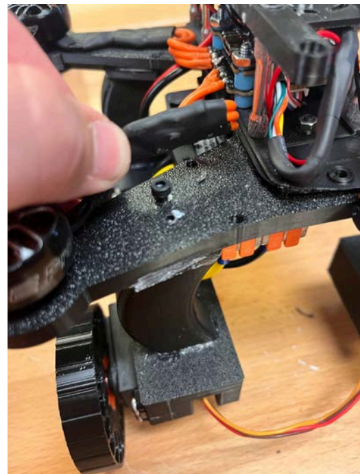
Made screw holes in the frame of the drone to be able to screw the legs into the frame
