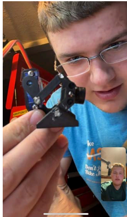
Working together on FaceTime to get the mount of the drone working, enabling the camera to move up and down
