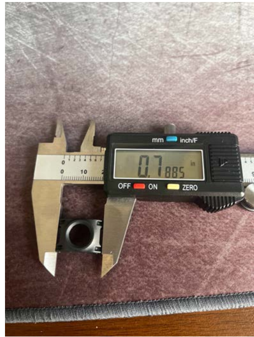
Another measurement of the camera's length instead of its width
