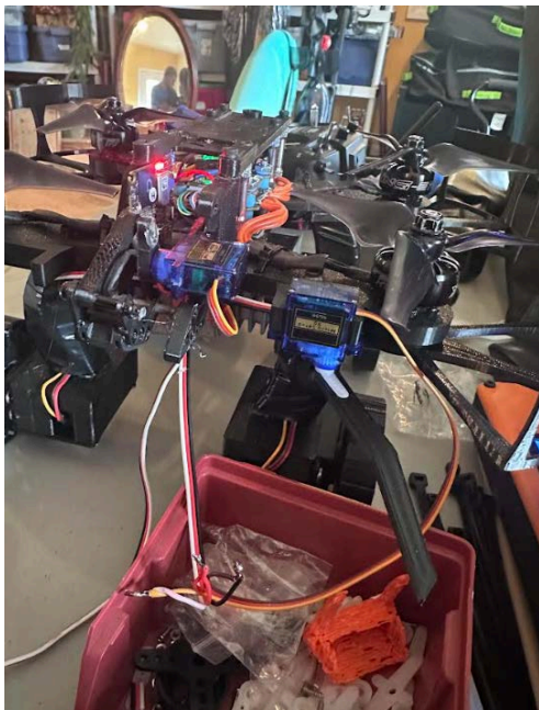
The servo is attached to the mount with the claw
