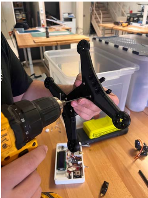
Constructing the 3D-printed frame of the new drone
