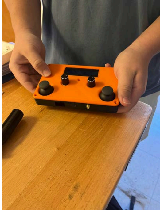
Placed and screwed on the lid, making sure the joystick and potentiometers sat correct
