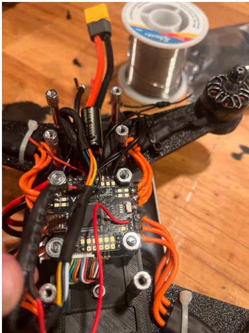
We soldered all of the motor wires onto the ESC and also soldered the 5v + wire on the flight computer to give the 04 air unit power
