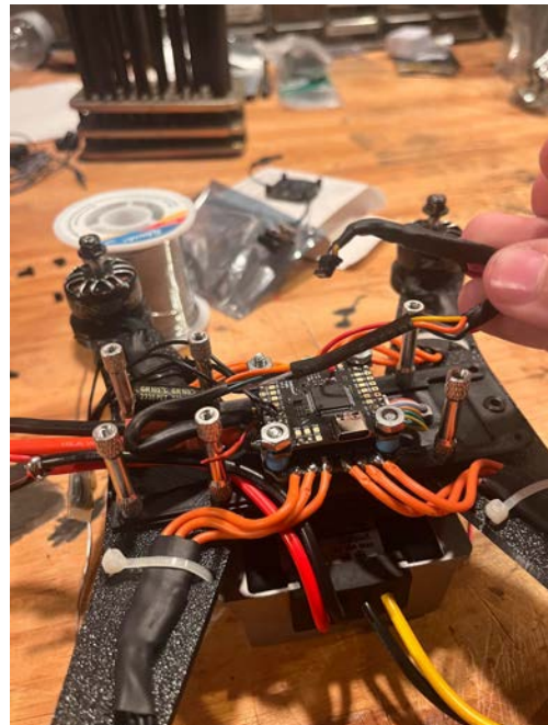
Another angle of the extension wire and all of the motor wires soldered in.
