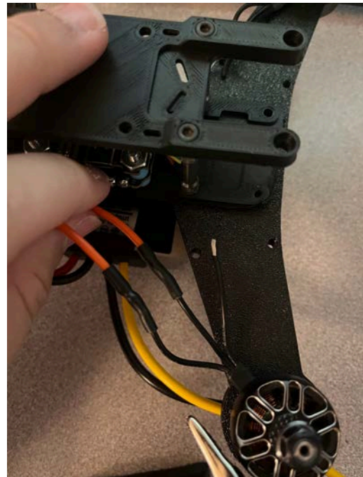
Began to fix up the motor wires to be soldered to the flight computer. Did this for all motors
