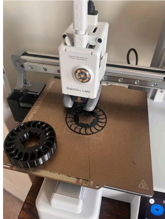
The tire is being printed using a specific filament called TPU to make it rubbery
