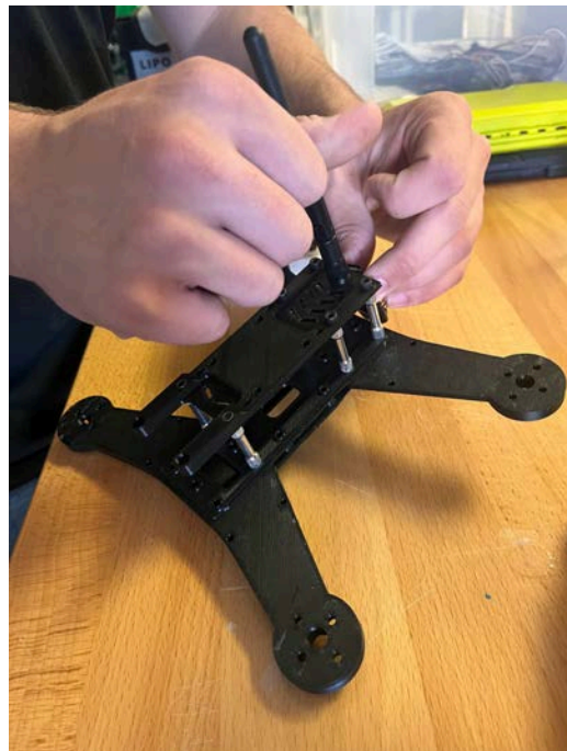
Attaching the top plate of the drone where the battery would sit.
