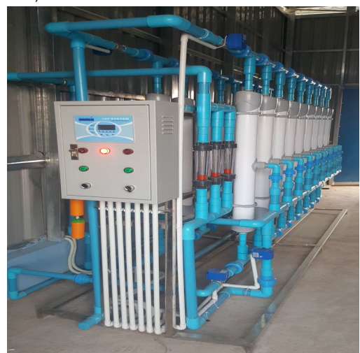
sUF-DECA-MMU-SDE-TWIN 12,000 l/h from riverwater
