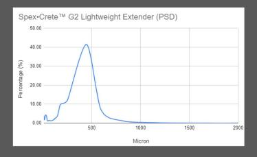
Spex•Crete™ G2 is a 100% recycled lightweight additive that is used to reduce the weight of your cementitious system. Spex•Crete™ G2 is free flowing and very easy to disperse into your system.
