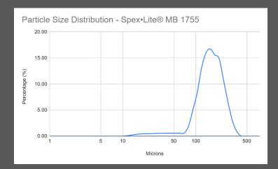
Spex•Lite® MB 1755 is a lightweight polymer microbead additive that is used to reduce the weight of your cementitious system as well as provide a very smooth surface profile.
