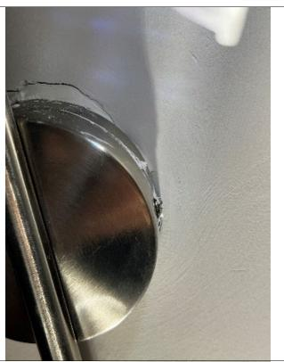
The external fan cover is scratched and dirty, this will need to be replaced.
