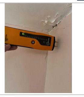
First image shows overview of internal window surround. Second image shows thermal image of cold spot. Third image shows the moisture meter picking up moister. External seals need replacing.
