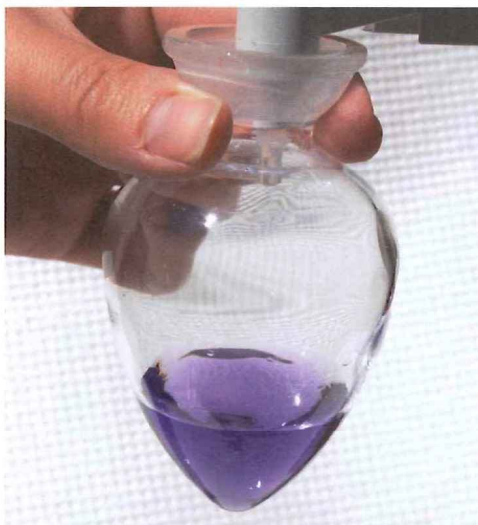
Figure V-e and V-f: In the aeration/oxidation method the sulfur dioxide is aspirated out of the wine sample before titration so the endpoint is not affected by the color of the wine. Before and after the endpoint are shown in figures V-e (left) and V-f (right).
