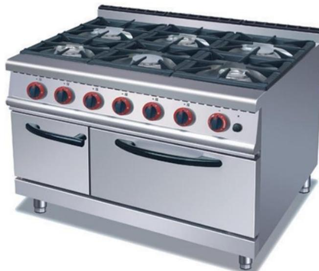
**JUSTA GAS range cookers**, with ovens underneath are high-performance, general-purpose ovens with linear burning and cast-iron pan supports on the hobs. The ovens use Italian gas valves that incorporate a microswitch flame failure feature, along with a further secondary safety flame-out device for added security. Each hob is also fitted with its own dedicated flame-out safety device. Oven choice of: 300x300(mm) or 400x400(mm) pan supports.
