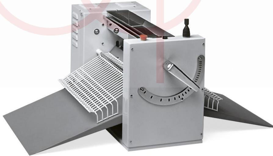
**Model GP 500-1000.** Category medium that benefits from more powerful 2-speed power units and higher dough handling capabilities. Ideal for pastry chefs and medium-to-large patisseries. GP 500 - 1000 has a 550 W motor, chain driven rollers and is capable of 8kg dough batches with a dough thickness adjustment range of 0.1 - 28 (mm).
