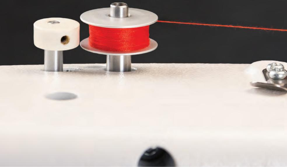
The Grace Q'nique machines features a **top-of-the-line bobbin system**, including a large M-class bobbin that is larger than standard domestic sewing machine bobbins, allowing you to quilt longer before having to refill it.
