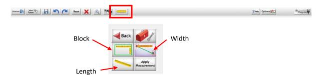
We have 3 ways in which we can measure something. Select the Block Icon and a rectangle appears, this allows us to measure both the height and width of a block and apply measurement.
