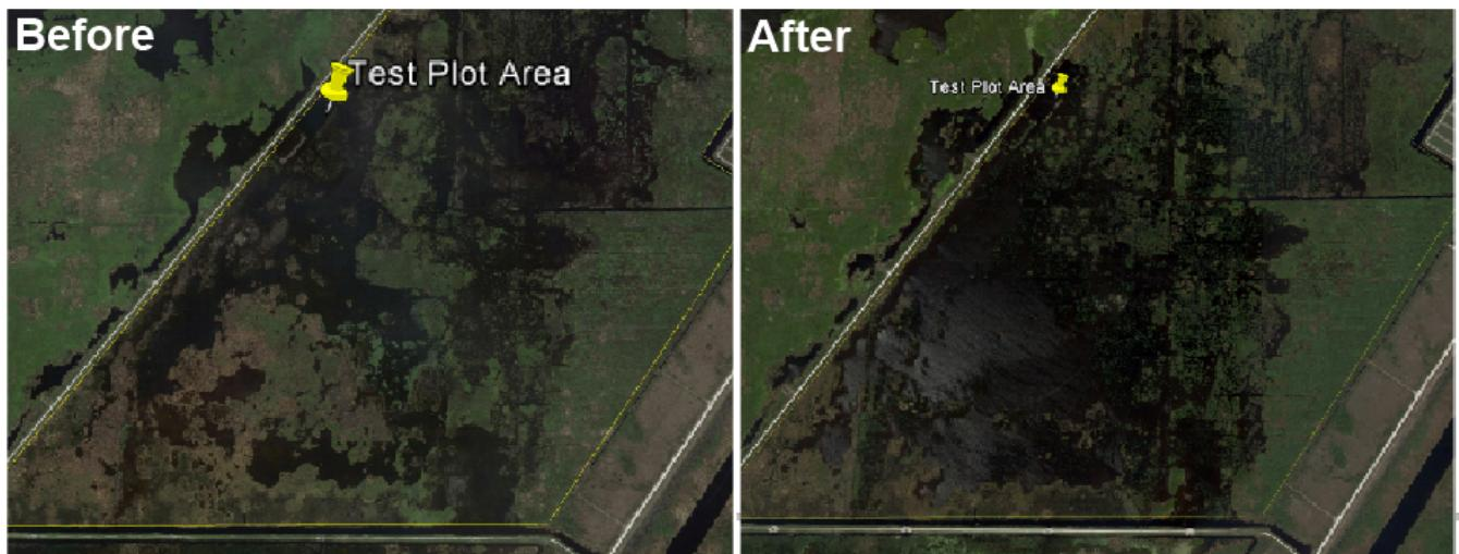
The clear water zones on the right hand side photo show the powerful change created by the Bio-Zyme dosing. The dosing does not injure plants but plants previously supported only by tussocks now lack support and move with the wind and flow. Plants anchored in firm substrate are unaffected.
