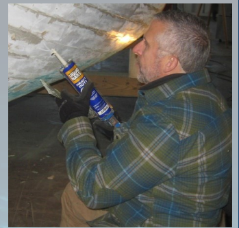
Howard using a product to fill in voids; John caulking the hull.
