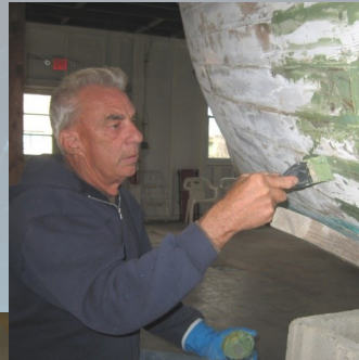
Howard using a product to fill in voids; John caulking the hull.
