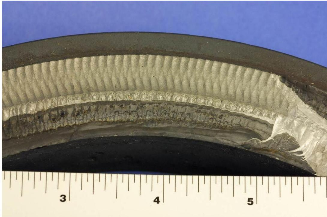
Fracture features consistent with separation at or near fusion boundary with base metal
