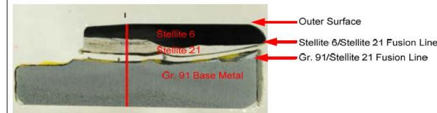
Study by Lolla, et.al., demonstrated that high hardness in diluted butter layer due to widespread formation of sigma phase
