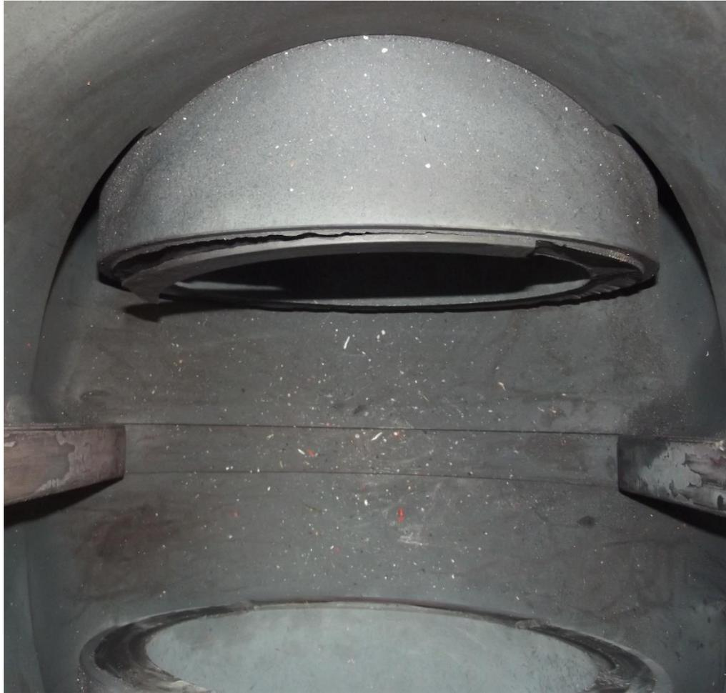
Numerous reports of separation of hardfacing materials from sealing surfaces in valves, such as seats and disks; loss of proper sealing and consequential damage from dislodged material has been a significant problem for plant operators
