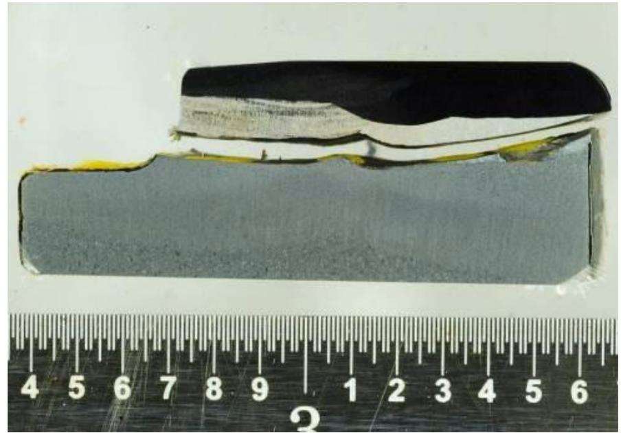
Fracture features consistent with separation at or near fusion boundary with base metal
