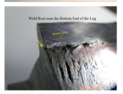
**Figure 3.** Shown are close-up views of the lug sample on the face-side (top photo) and root-side (bottom photo) of the weld.
