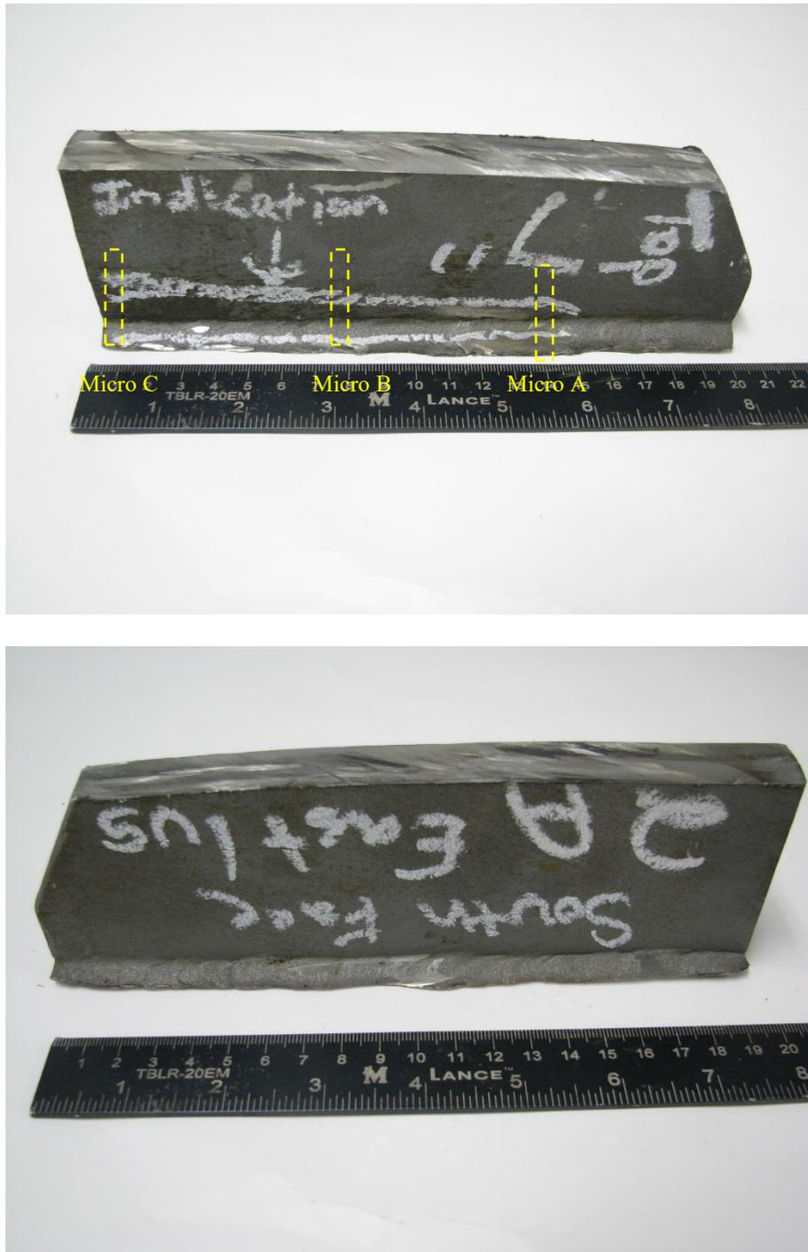
**Figure 2.** Shown are the general features of the lug sample in the as-received condition; the approximate locations from which the metallographic specimens were removed also is indicated in the top photo.
