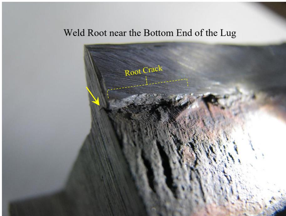
**Figure 3.** Shown are close-up views of the lug sample on the face-side (top photo) and root-side (bottom photo) of the weld.
