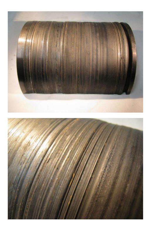
**Figure 4.** Documenting score marks and deep gouges visible on the external surface of the sleeve where it was in contact with the internal surface of the bushing.
