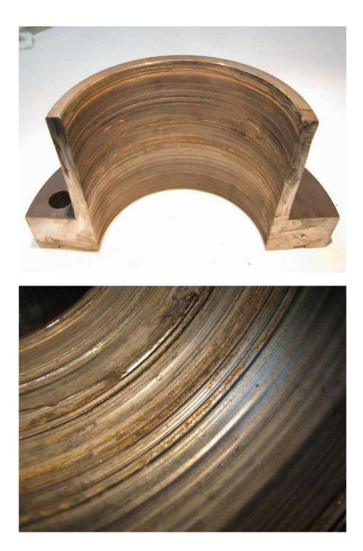
**Figure 5.** Showing score marks and deep gouges that were visible on the internal surface of the bushing where it was in contact with the outer surface of the sleeve.
