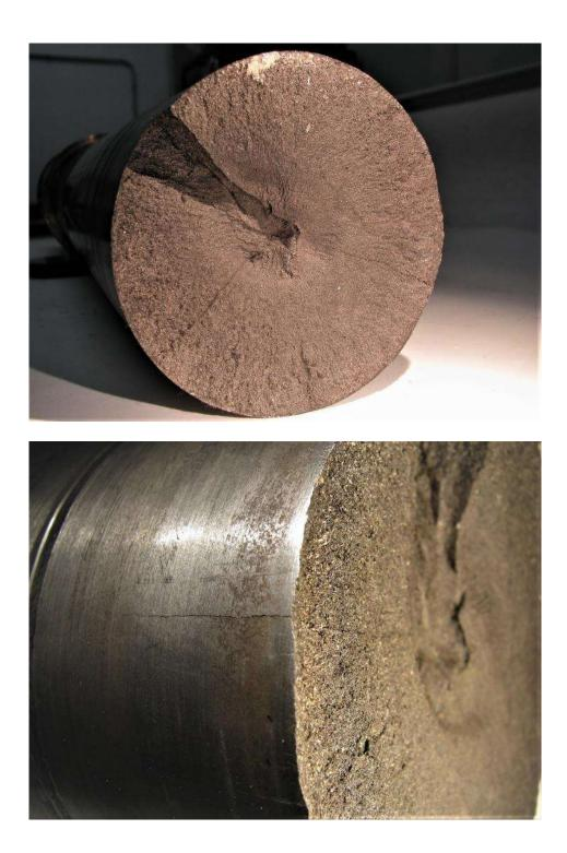
**Figure 5.** Documenting the general appearance of the primary circumferential fracture in the shaft and showing one of the secondary axial cracks that straddled the primary fracture. Both the axial and circumferential fractures were non-ductile in character.
