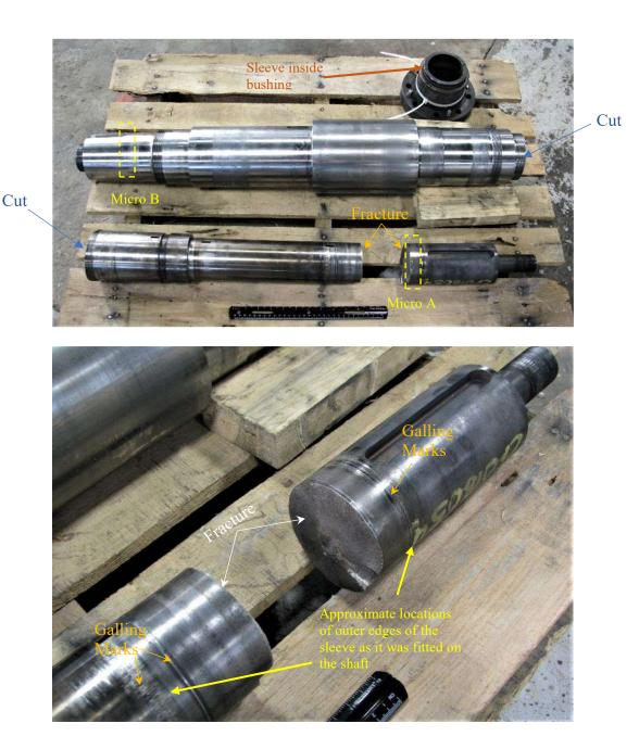
**Figure 1.** In these photographs, the various pieces of the boiler circulation pump involved in the failure are shown as they appeared when received by ATC-CES. The location of the circumferential fracture in the shaft and the estimated position of the sleeve and bushing on the shaft are indicated. Note the discoloration of the shaft surface at the failed end of the shaft.
