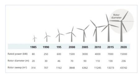
Above: The leap from 8 MW to 18 MW turbines has occurred in significantly less time than it took to go from 3 MW to 8 MW. Only five years ago, 8 MW machines were the largest turbines in the industry. But today, manufacturers are moving up to the 18-21 MW threshold, with plans in place for turbines to grow bigger still, reaching the height of a 70-story building (source: GCube)
