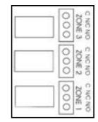
Maximum switch voltage is 240v and maximum switch current is 8 Amps.
