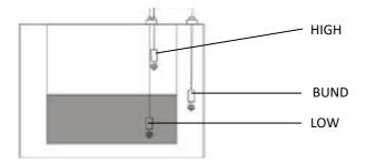
The probe wired to the **HIGH** connection is positioned at the topmost part of the tank and is used to alert that an overfill has occurred. The probe wired to the **LOW** connection should be positioned near the bottom of the tank to indicate a low-level. The **BUND** probe is placed between the two tank 'skins' and is used to quickly alert of any leaks.
