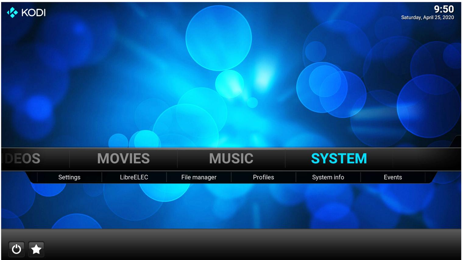
If not, use remote or connect mouse and keyboard and go to: System > Settings > System > Settings level and change it to "Expert".
