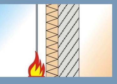
Proper design rear ventilated facade is a fire safe.
