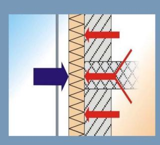
In wintertime exterior insulation layer preventing the escape of heat from the inside of the building.
