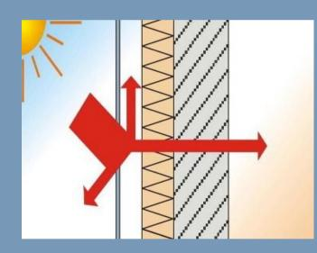
The cladding protects enclosure walls against the direct sun. The air cavity between insulation and cladding created a "chimney effect" which cools the building and helps to save energy in the summertime.
