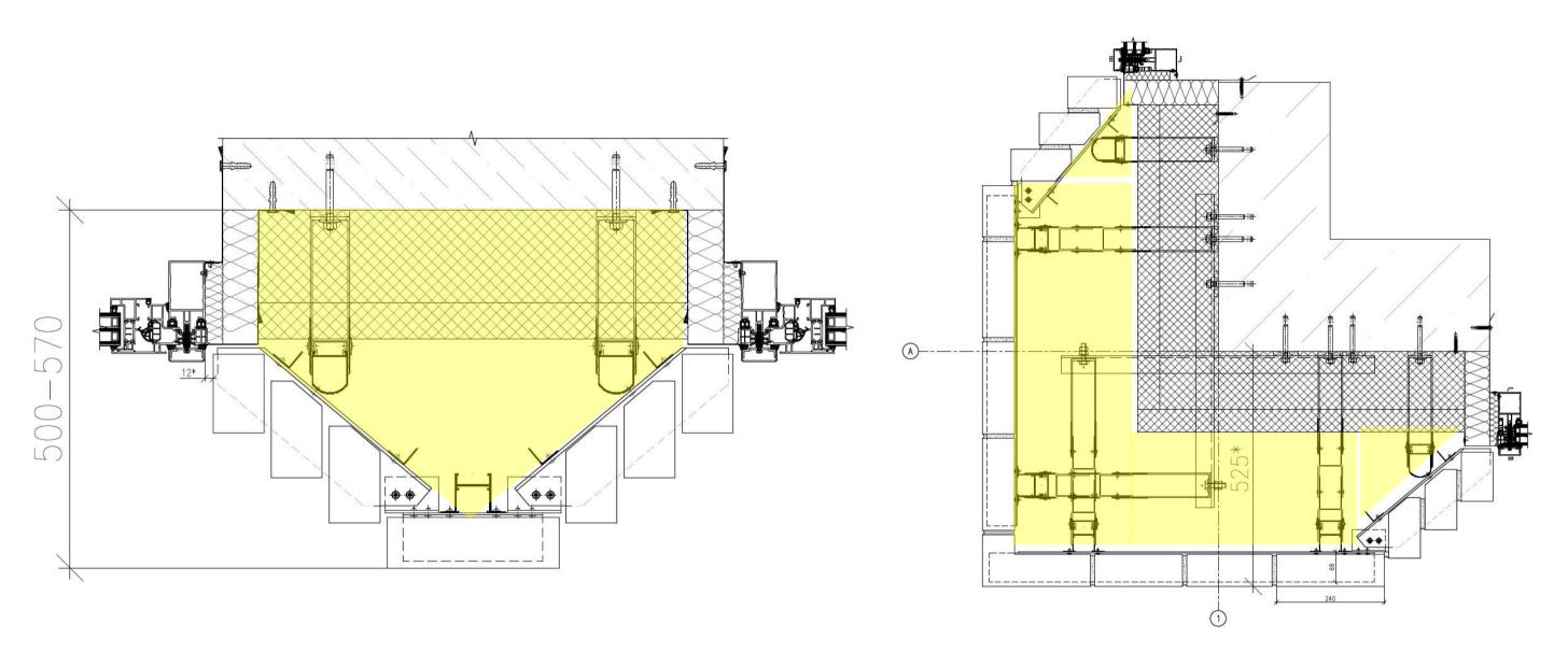
Using heavy duty vertical profiles with combination of "U" shape wall brackets can accommodate any loads and use in complex facade shapes
