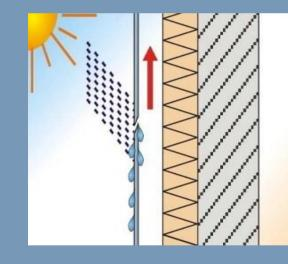
The rear ventilated facade allows water to penetrate through open joints but not more than 5% Effective ventilation behind the cladding effectively removing any water inside of facade system.
