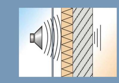
The rear ventilated facade consists of several layers including fibre insulation which helps to reduce a sound level up to 15 dB.
