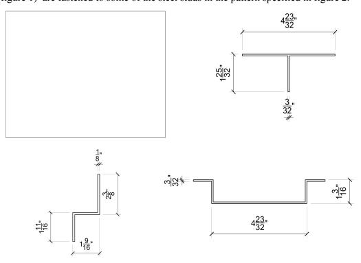
**Figure 1:** Wall bracket (top left) 100mm deep 3mm thick bracket 85mm long aluminum grade 6063T6. Horizontal support section (bottom left) 40mm deep 3mm thick zed section aluminum grade 6063T6. Support bracket (bottom left) 120x45x2mm T section 60mm long aluminum grade 6063T6. Vertical support section (bottom right) 30mm deep 2mm thick top-hat section aluminum grade 6063T6
