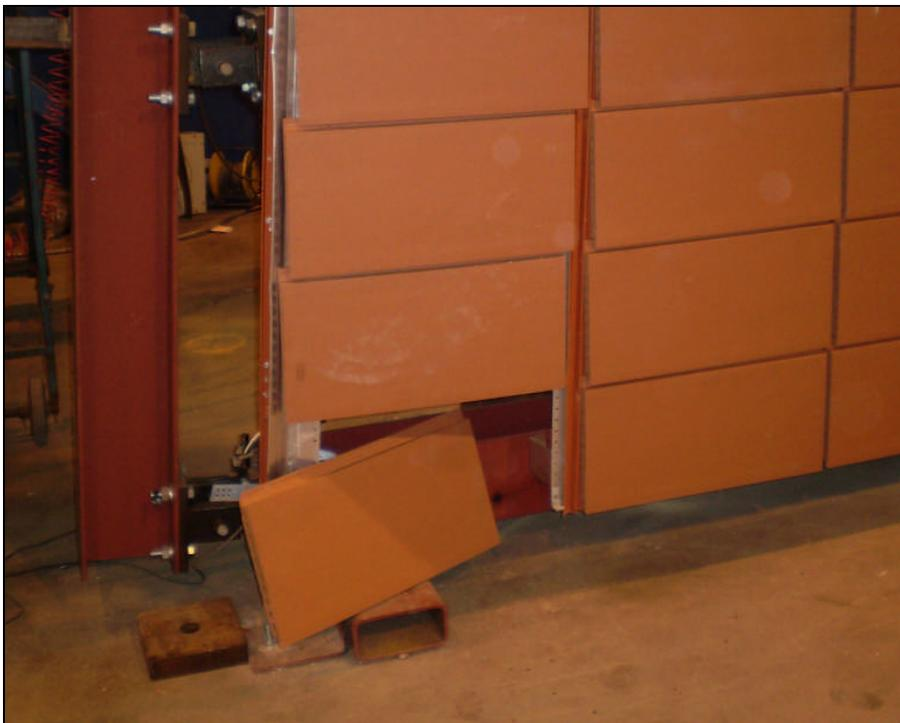
Argeton sample 3 failure after testing.
