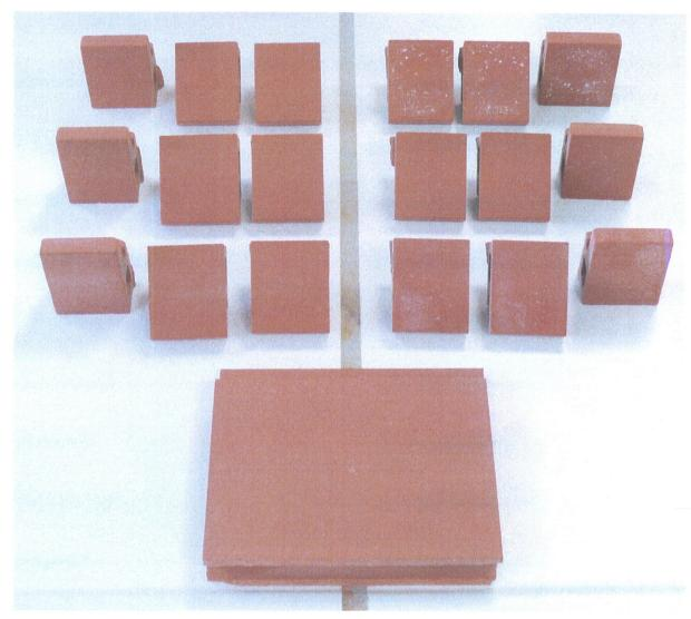
Fig. 1:Each 3 of the 6 specimens from the resistance testsLeft side:"low concentration (L)", from top to bottom, test run 1, 2, 3Right side:"high concentration (H)", from top to bottom, test run 1, 2, 3
