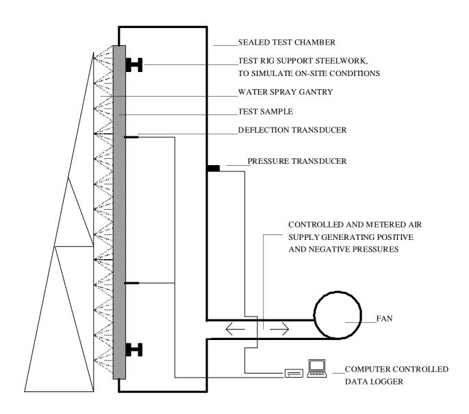
SECTION THROUGH TEST RIG
