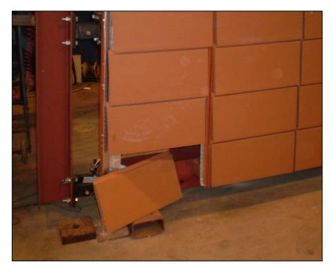
Argeton sample 3 failure after testing.
