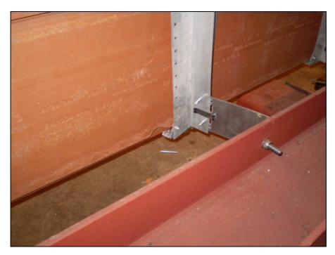
Argeton, sample 1 – Damaged clip and tile after testing
