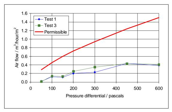
Air infiltration test results
