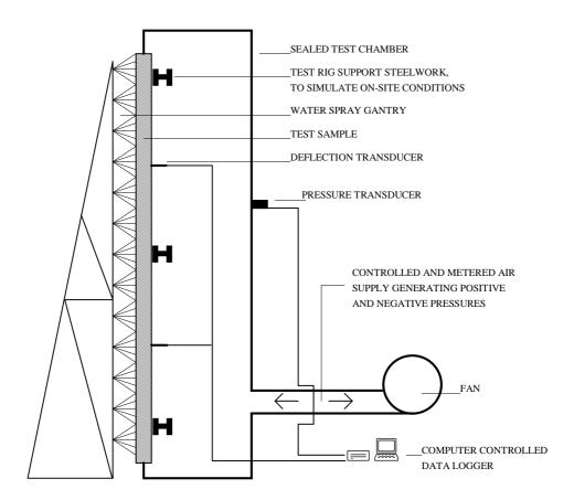
SECTION THROUGH TEST RIG
