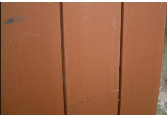
SAMPLE AFTER 350 Nm SOFT BODY IMPACT TEST
