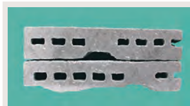
Hollow core CERACLAD panel after 600 freeze/thaw cycles. Extruded panel demonstrates its strength even in cold climates.
