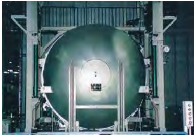
Autoclave for curing CERACLAD panels
