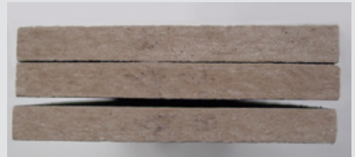
CERACLAD after 100 cycles - Hollow core demonstrates its strength even in cold climates
