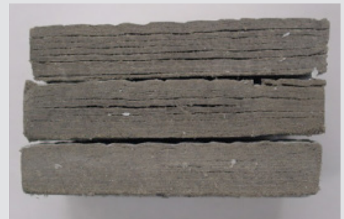
Typical fiber cement products after 100 cycles
