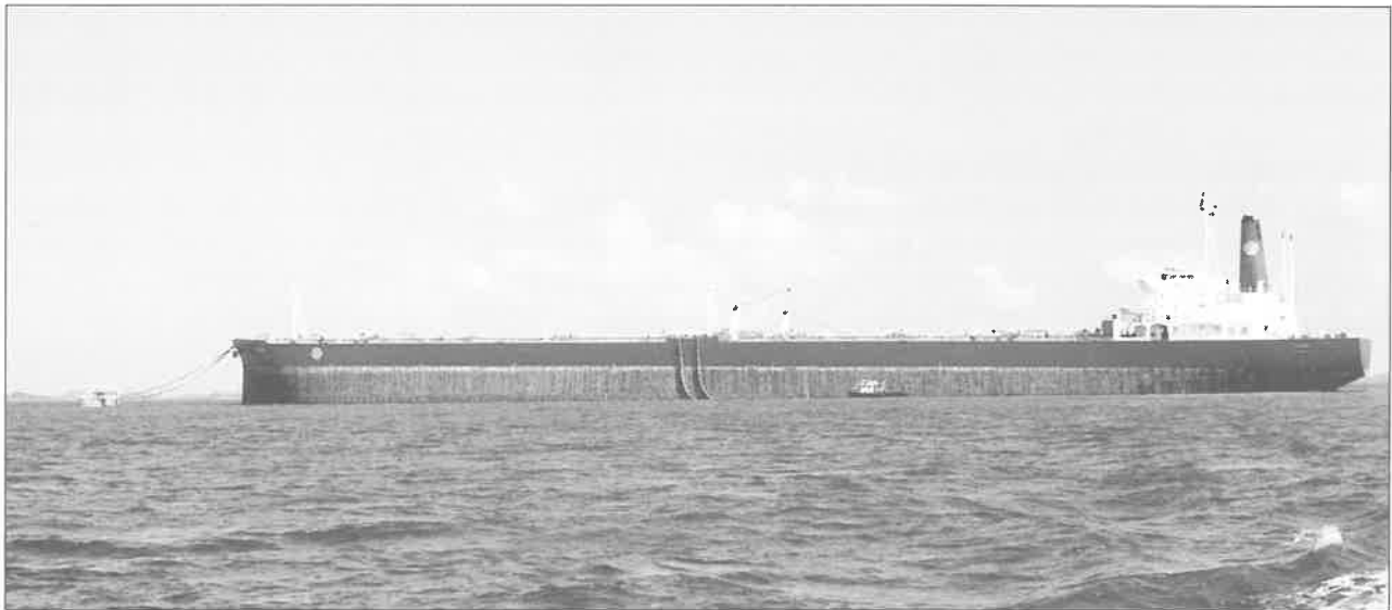
49. Ultra Large Crude Carrier, ULCC, lying to a Single Buoy Mooring (SBM).
