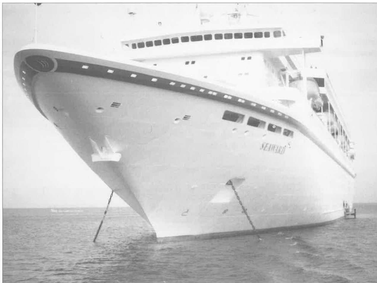
48. Class 1 Passenger Cruise Liner 'Seaward' with both anchors deployed off Cozumel Island, Mexico. Stem anchor also visible.
