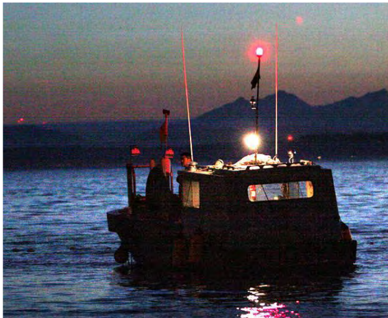
These photos point out the red over white lights and bouy balls, which include a flashing jack light to identify the end of the net.
