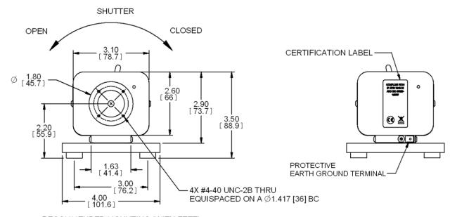
RECOMMENDED MOUNTING (WITH FEET) 4X  $\varnothing$ .25 GROMMET THRU HOLE
