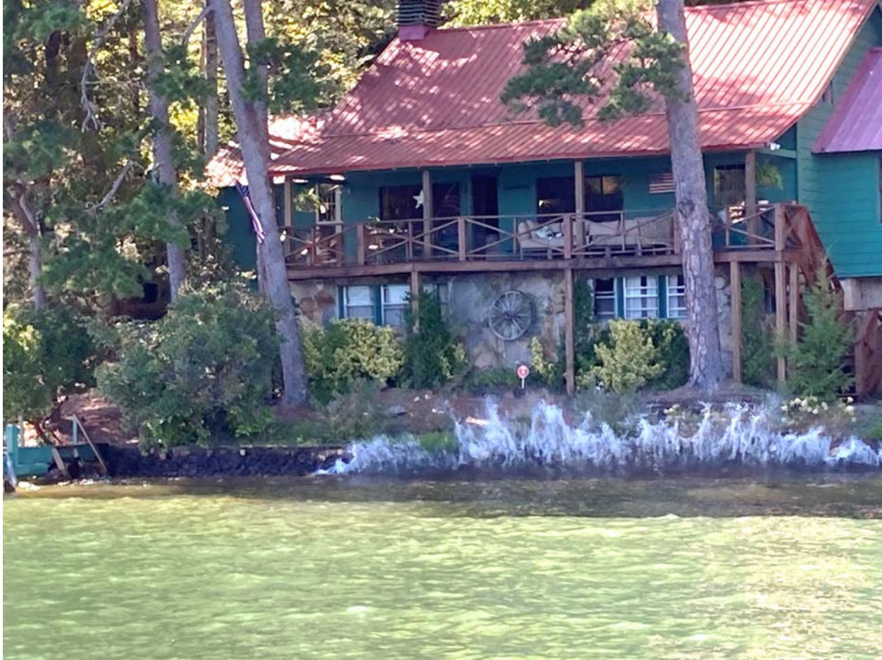
Figure 3-3. Example wave run-up from wakesurfing wave impact during field testing
