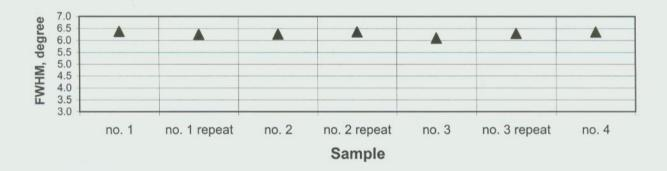
FWHM - Full Width at Half Max... measure of peak width.0 Stress Fe Powder Performance Verification Check Measured :0.7 +/- 0.5
