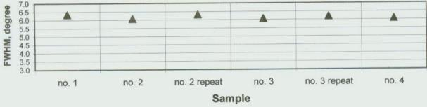
FWHM - Full Width at Half Max ... measure of peak width. 0 Stress Fe Powder Performance Verfication Check Measured : 0.6 +/- 0.5
