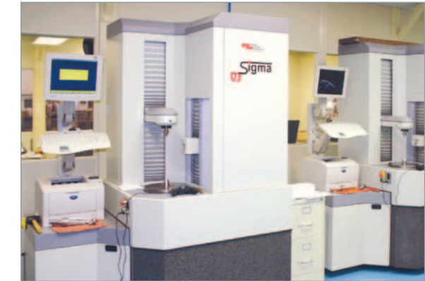
M & M 400 CNC gear inspection systems in temperature and humidity controlled room.
