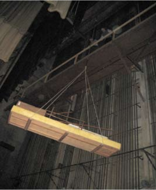
The 32' Wood Diaphone Set. The six pipes each play two notes by opening a trap door at the top.
