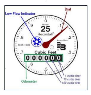
The odometer shows how many gallons or cubic feet have been used and the dial shows how many tenths of a gallon/cubic feet have been used. The reading for the meter above is 0.13 cubic feet. To check water usage, read your meter at two different times and subtract the numbers:
