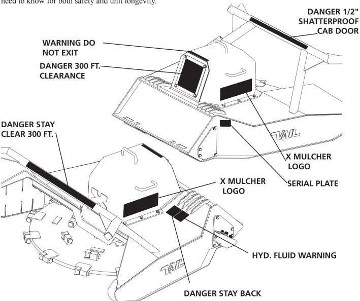
**IMPORTANT:** Keep all safety signs clean and legible. Replace all missing, illegible, or damaged safety signs. When replacing parts with safety signs attached, the safety signs must also be replaced.
