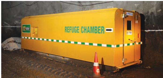
Hindustan Zinc always endeavors to support the occupational health and safety of employees working underground. Therefore, as a safety initiative for underground mines, HZL installed a Refuge chamber which provides a place of safe refuge (protection) and fresh air, in case of emergency situations like fire, rock fall and blockage of escape routes etc. Refuge chamber can accommodate up to 20 persons and has a life support back up of 36 hours.
