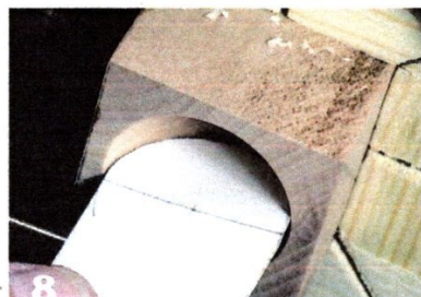
8 A template made of cardboard functions as a depth gauge as well as a shaping guide.
