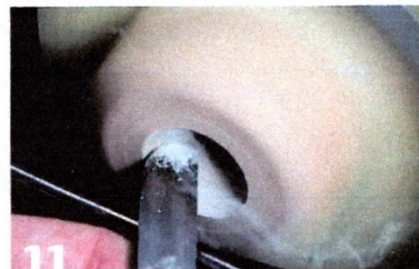
11 Hollowing proceeds quickly and cleanly with a negative-rake scraper.
