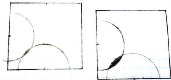
Figure 1 Use graph paper to plan the size of the bowls, and the corresponding holes between them. The area of overlap determines the size of the holes between the various faces.
