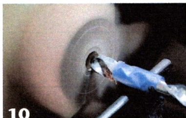
10 Easily establish the depth with a marked drill bit.
