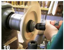
With a 3"-diameter soft disc, sand the interior of the bowl.
