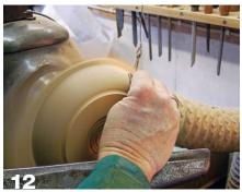
Sand what you can on the bottom now, as you won't be able to come back to it later. Sand the overhanging flange of the rim with the lathe off.
