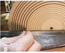
Create well-defined details by pushing a thin wedge of dark wood into the spinning grooves. This works most dramatically on lighter-colored woods but can be a subtle accent with darker woods, too.
