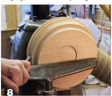
With the lathe stopped, it is easy to see how the offset mounting affects the cutting of the platter's rim.
