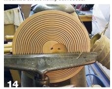
Although it looks odd, the hole on the right is the new center of the platter.
