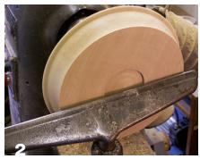
Flatten the bottom, make a recess for the chuck, and establish a rounded edge.
