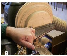
Cut away the first recess and make a flat bottom. Then mark for the new recess that will be centered on the new axis.
