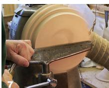
Cut away the bulk of the off-center rim. Work from the outside in stages, pivoting the gouge into the blurred spinning wood.
