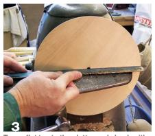
Turn a flat top to the platter and check with a straightedge.
