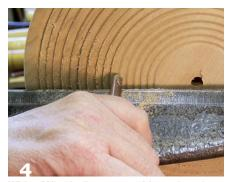
With a  $\frac{3}{8}$ " spindle gouge, add a series of beads to the platter.
