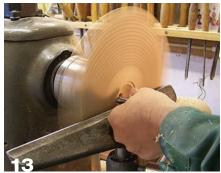
Start to hollow out the platter, which is mounted on the newly cut recess.
