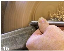
To begin hollowing, hold the flute at 3 o'clock. The bevel will head straight into the spinning beads. Once safely past this point, rotate the tool to a more open position.
