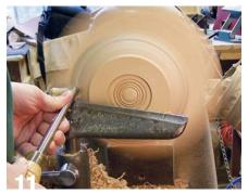
Make your final cuts to the bottom of the rim and bowl section of the platter.
