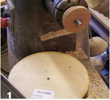
Start with a sound blank, roughly 10" in diameter and 1½" to 2" thick. Mount the stock on a screw chuck like normal.
