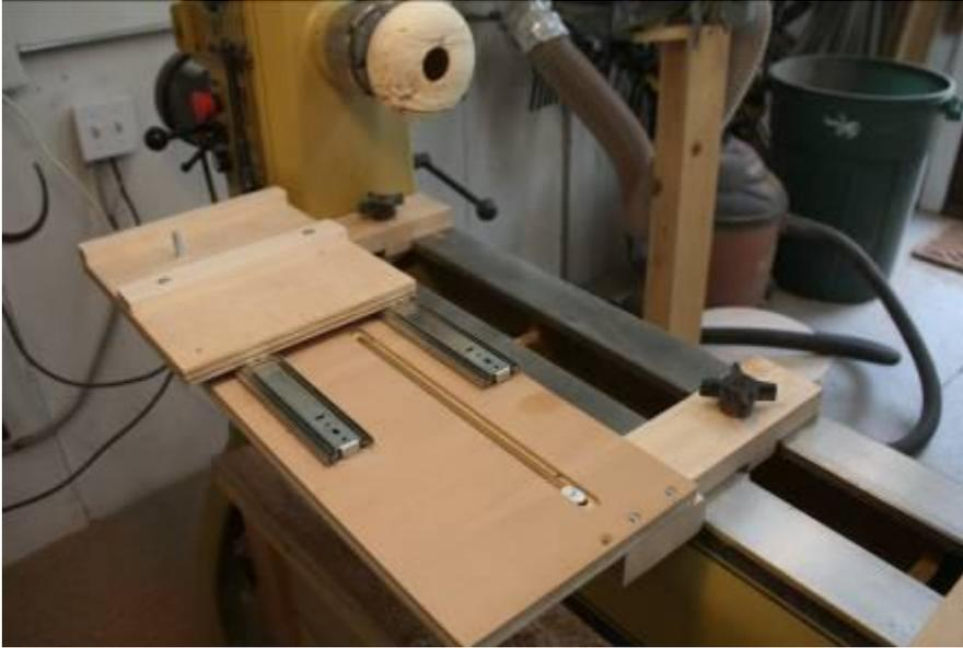
Sliding platform locked in place. Note drawer guides to align fixture.
