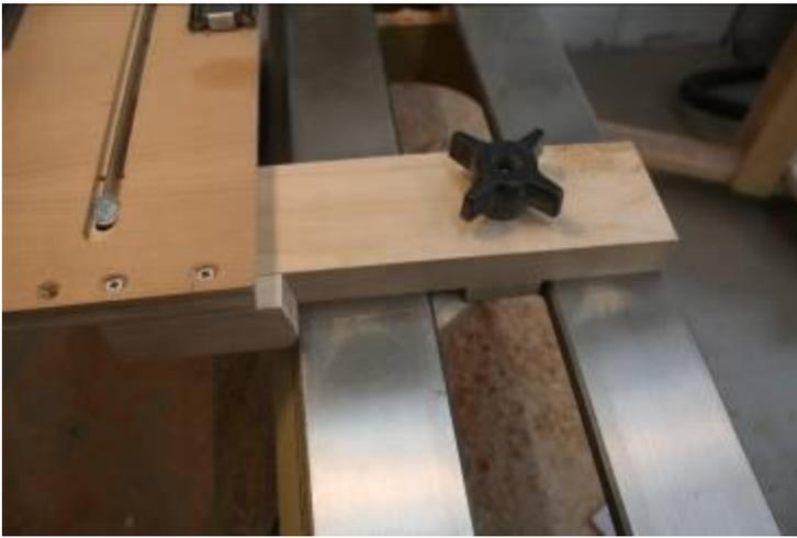
Locking mechanism for platform, right side
