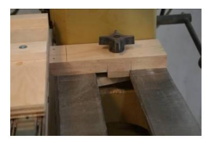
Locking mechanism for platform, left side
