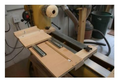
Sliding platform locked in place. Note drawer guides to align fixture.
