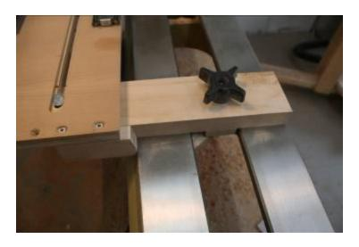
Locking mechanism for platform, right side
