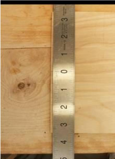
I then measure the width of the carrier plate, divide that number in half, and put a pencil mark at the halfway point. I find it easier to use a center zero ruler to find the center point than having to figure half of, say  $7 \frac{5}{32}$ " for example. No math is necessary.
