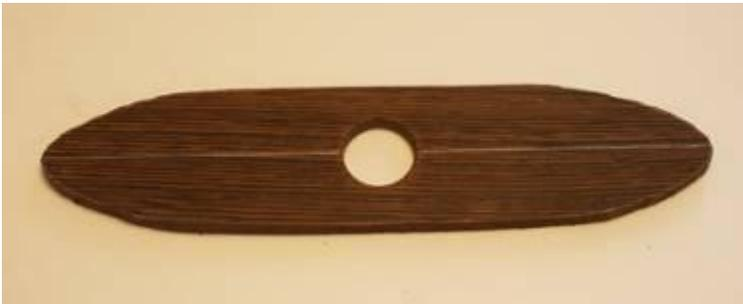
The hole for the top finial has been drilled. The measurements I took earlier will insure that the hole will be in the center of the finished top. Don't make the hole wider than the distance between the 2 sides of the vessel at its center point.
