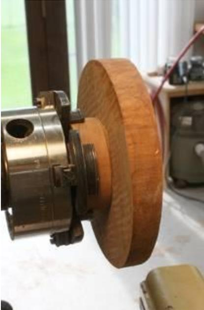
This is a side view of the blank mounted on the lathe. It's important to note that the side of the blank facing the headstock will become the outside of the vessel, the opposite of the way you normally turn a bowl.
