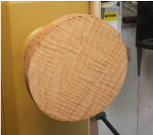
The blank has been mounted to the lathe. In this case, I'm using a solid piece of wood rather than gluing together 2 separate pieces. I've used double sided turners' tape to attach the blank to a waste block. This allows me to use the entire thickness of the blank, in this case about  $\frac{7}{8}$ ". Normally I use a waste
