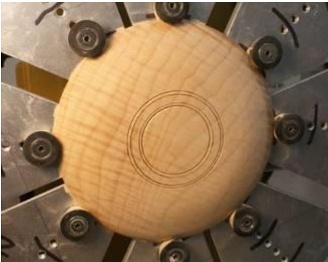
I've added a set of grooves and lines. The grooves are an incised detail and the lines mark the area that'll be textured. I use a parting tool ground down on the sides to make it very thin, around  $\frac{1}{32}$ " , where it enters the wood. You can use a skew instead, but there's less chance of the tool catching and skating along the surface with the thin parting tool.
