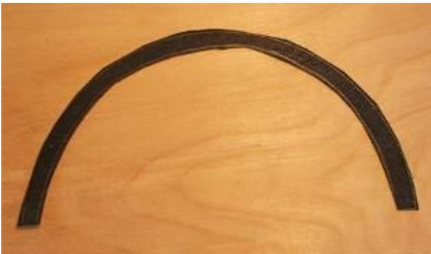
This is a piece of black dyed veneer I cut to act as a detail strip where the 2 halves are joined. This strip also helps conceal the differences in grain pattern from one side to the other. On larger pieces, I'll use either multiple layers of veneer or solid wood cut to 1/16" or so thickness.
