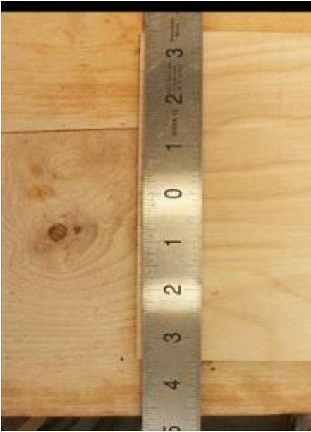
I then measure the width of the carrier plate, divide that number in half, and put a pencil mark at the halfway point. I find it easier to use a center zero ruler to find the center point than having to figure half of, say  $7 \frac{5}{32}$ " for example. No math is necessary.
