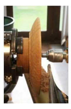
Here I've roughed out the outside of the vessel, up the point where it reaches the mounting block.
