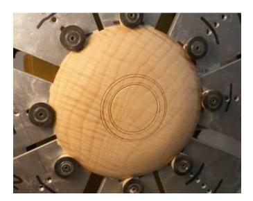
I've added a set of grooves and lines. The grooves are an incised detail and the lines mark the area that'll be textured. I use a parting tool ground down on the sides to make it very thin, around 1/32", where it enters the wood. You can use a skew instead, but there's less chance of the tool catching and skating along the surface with the thin parting tool.
