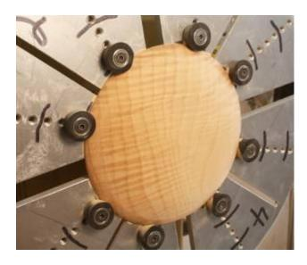
The outside of the vessel has been turned to its final shape. The goal is to maintain an even curve around the bowl since it'll be visible once the top is glued on.
