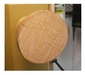
The blank has been mounted to the lathe. In this case, I'm using a solid piece of wood rather than gluing together 2 separate pieces. I've used double sided turners' tape to attach the blank to a waste block. This allows me to use the entire thickness of the blank, in this case about 7/8". Normally I use a waste
