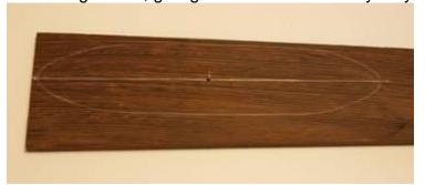
The outline of the top has been traced on the blank, here a 1/8" piece of wenge. I've drawn a line through the center, using marks I made where the center spline is located. I divided the line in half and marked where the center of the hole will be.
