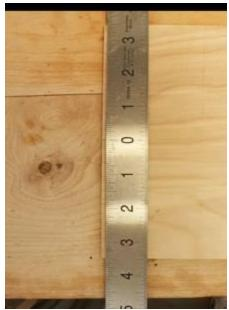
I then measure the width of the carrier plate, divide that number in half, and put a pencil mark at the halfway point. I find it easier to use a center zero ruler to find the center point than having to figure half of, say 7 5/32" for example. No math is necessary.
