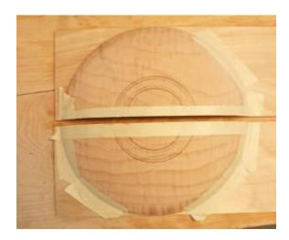
The vessel has now been cut in half. It's important to feed the carrier through the saw a steady rate to insure that the cut edges will be perfectly straight. If you change feed rates or stop partway through, you can get a slight dip in the cut edge. Or worse, you could get a nasty kickback. There's no danger of kickback with a bandsaw, but it's important to properly tune the saw to avoid blade drift. You want the cuts to be as centered and straight as possible.
