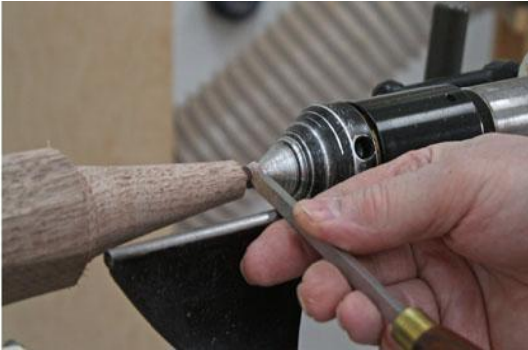
3. Shaping the end cup with a small skew.
