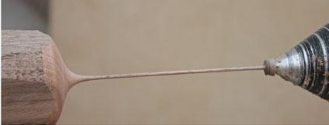
8. The stem turned and sanded at its final length.
