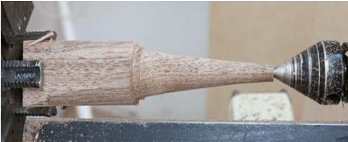
2. Blank turned with tapered cone at end.
