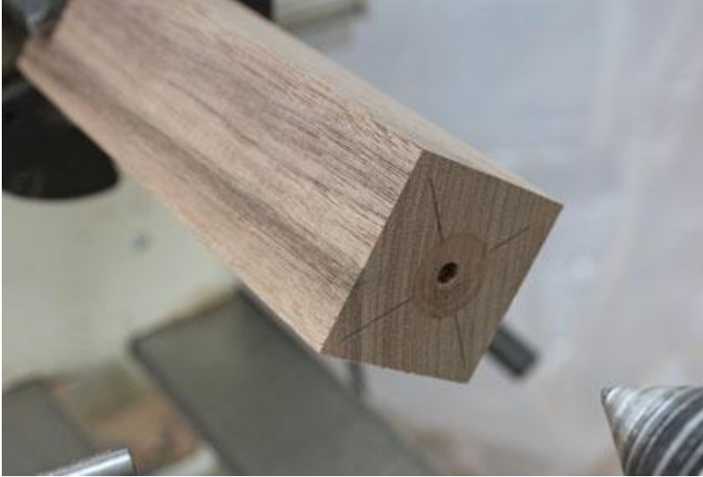
1. Blank mounted with hole and recess in end
