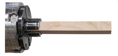
Two ways to mount your blanks in a chuck. If you do not have pen jaws you can remove the jaws and use the slides to hold the piece. It is not as secure as pen jaws, but if you don't get
