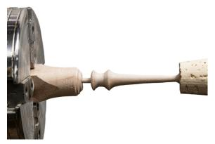
Finish turning the upper portion, including the 1/8" tenon. I try to make sure it is a "fat 1/8 since there is no way to test fit before cutting off. I would rather spend a few minutes making it fit than trying to add wood back. I do not
